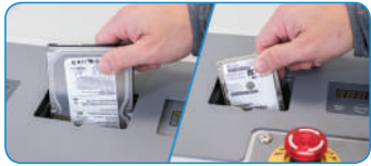
Separate feed openings for 3.5" and 2.5" drives
