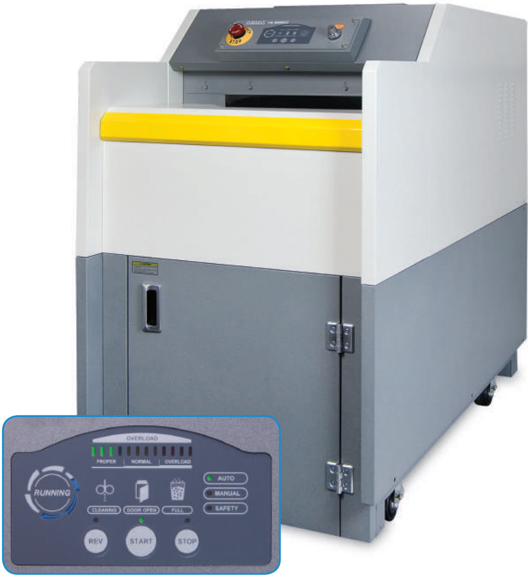
Control Panel includes LED load indicator, safety key and emergency stop button
