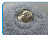
Optical media particles: <math><1.5\text{mm}^2</math>, nearly as fine as salt
