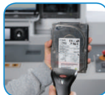
Barcode reader documents hard drives being shredded
