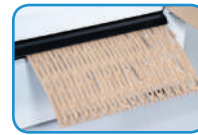
Perforates and trims cardboard in a single pass
