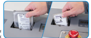
Separate feed openings for 3.5" and 2.5" drives
